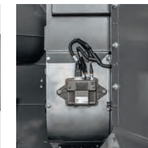
Fewer and shorter stops for unloading are soon reflected in a greater daily yield – sensors for yield and moisture and a grain quality camera are fitted to the elevator. The data is accurate to 98%, and applied with the VarioDoc ISOBUS standard, live yield mapping and IDEALharvest™.
