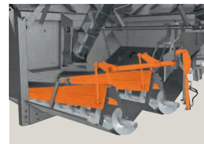
Cover flaps above the augers in the grain tank floor control the discharge speed in five positions.
