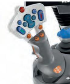
The optional multi-function joystick also features buttons to control two hydraulics valves.
