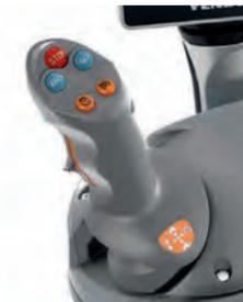
Use the joystick (fitted as standard) to control the speed, cruise controls, engine speed memory and headland management.
