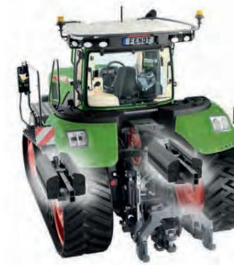
2,690 kg: 64 weights on the inside and outside of the undercarriage (32x per tread)
