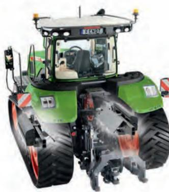
1,345 kg: 32 weights on the outside of the undercarriage (16x per tread); dirt guard on the inside
