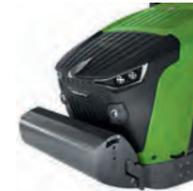
Front weight carrier with 330 kg and slot-in weights with a total of 1,645 kg
