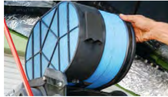
The air filter is easy to replace and has a dirt sensor, which provides information on the filter effect.
