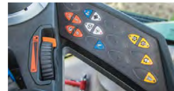
Adjust the gearbox, hydraulic and PTO settings using the membrane keys in the armrest.
