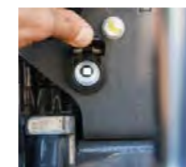
■ The 12 V connection at the rear of the machine supplies power to the external consumers.
