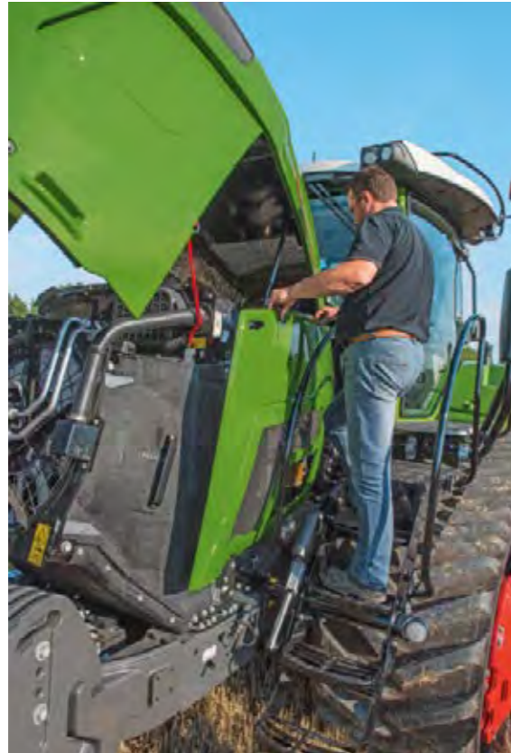
The engine compartment is very accessible, with removable side panels.
