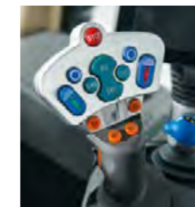
The optional Profi joystick also features buttons to control two hydraulics valves.
