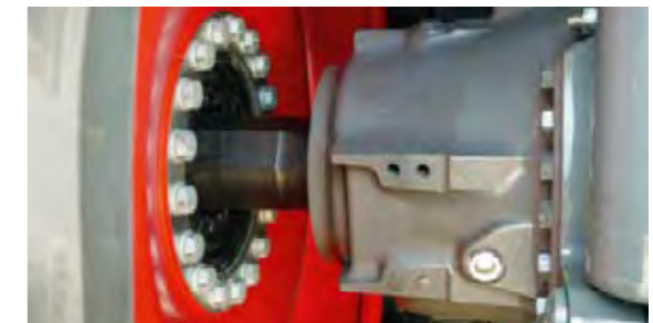
The durable rear axle is built for the longest service life. The internal oil balance can be easily checked through the inspection gauges.
