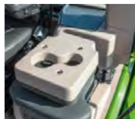
■ The instructor seat with seat belt serves as a bottle holder when folded down.
