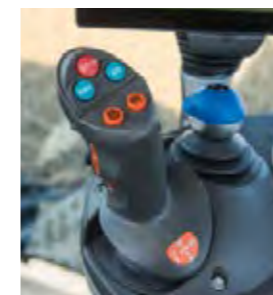
Use the multi-functional joystick (fitted as standard) to control the speed, cruise controls, engine speed memory and headland management.
