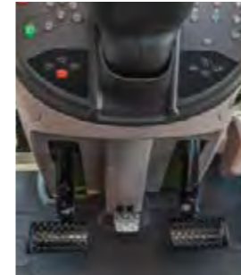
Adjust the position of the steering wheel with the foot pedal.
