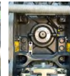
Select between two PTO speeds: 1000 and 1000E.
