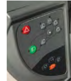
Activate the headlights and working lights on the left side of the instrument panel.
