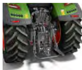
Rear linkage with ball ends and rub blocks
