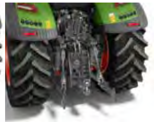
Rear linkage with quick-catch hooks and rub blocks (AU, South Africa, Eastern Europe)
