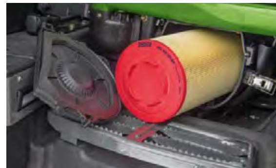
The cab filter is easily accessible in the door area and can be easily cleaned when necessary.
