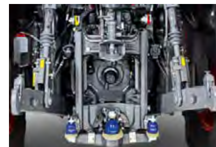
The lower links on the rear linkage can be folded up into parking position, so that there is more space for the drawbar.
