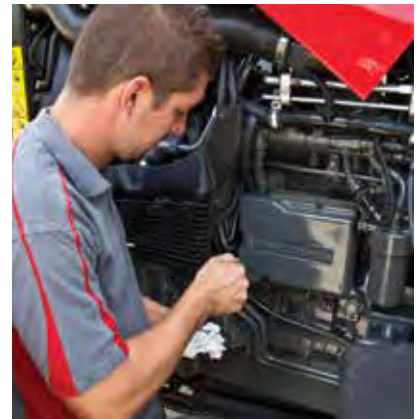
The waisted bonnet and front axle design ensures comfortable access to the engine oil filters and oil dipstick
