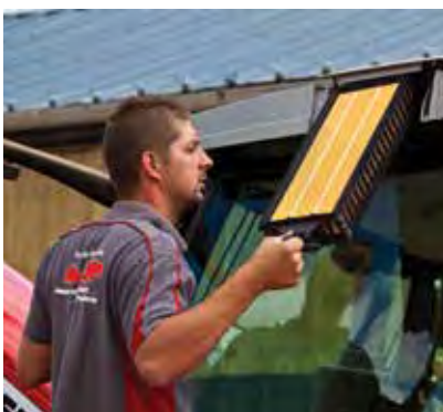
The cab air filter can be removed easily for cleaning
