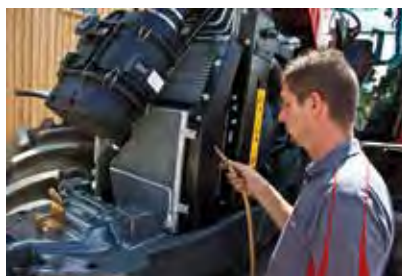
Plenty of room to access radiators for cleaning
