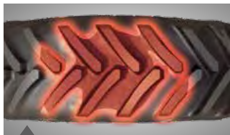
650/85R38 2 pairs of lugs Smaller contact point, weight is distributed unevenly resulting in more compaction.
