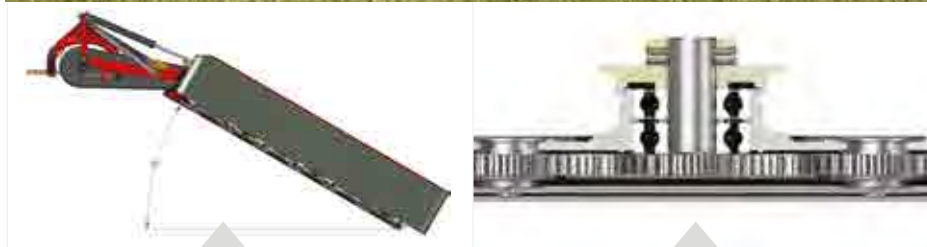
Side hitch attachment: makes mowing possible on sloping terrain
